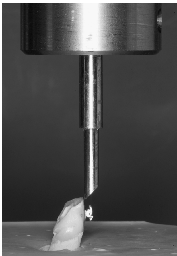
Figure 1 Experimental setting: a chisel-shaped rod applied the shear force as close to the bracket–tooth interface as possible. The bovine teeth were embedded in dental stone.
